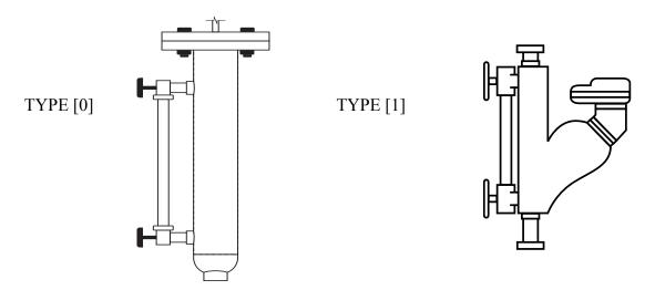
It is extremely important that the type of level control supplied and type listed in the solid state controller be the same. The generator is factory shipped with matched types.
